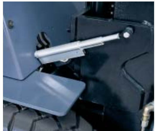
Tilt indicator mounted between cowl and mast.
