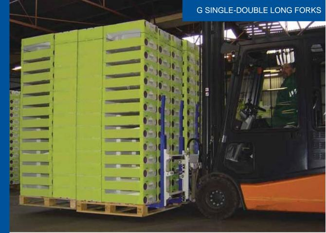
Allows the handling of up to four pallets at a time.
