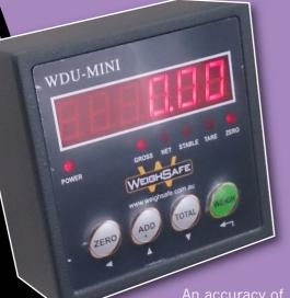
The WEIGHSAFE WDU MINI is a compact micro-processor based unit connected to the hydraulic lifting system found on lift trucks or similar machines. A load is placed on the forks and is then accurately weighed by measuring the hydraulic pressure required to raise the load. The hydraulic sensor measures pressure and converts it to an electronic signal which is displayed on the WDU MINI Monitor.
