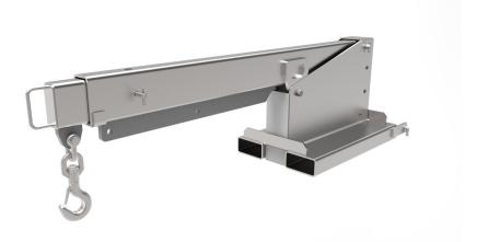
Note: All lift truck attachments affect the safe working load of a lift truck. End users should consult their lift truck supplier to ensure the lift truck is rated for use with these attachments. In the case of a slung load when lifting a jib attachment, the net lifting capacity should be 0.8 times the rating of the lift truck to allow for the swinging load. Please consult your local lift truck dealer.
