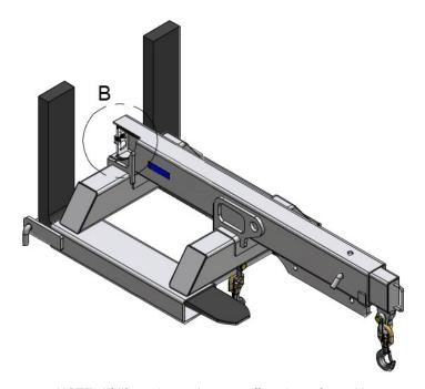
NOTE: All lift truck attachments affect the safe working load of a lift truck. Users should consult their lift truck supplier to ensure the lift truck is rated for use with these attachments. In the case of a slung load when lifting a jib attachment, the net lifting capacity should be 0.8 times the rating of the lift truck to allow for the swinging load. Please consult your local lift truck supplier.
