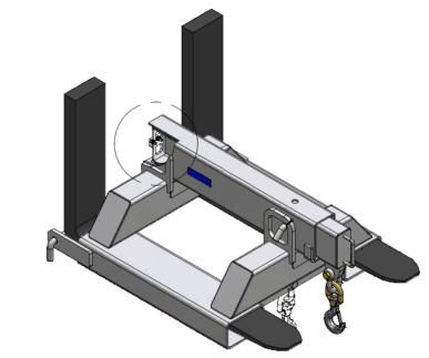
NOTE: All lift truck attachments affect the safe working load of a lift truck. End users should consult their lift truck supplier to ensure the lift truck is rated for use with these attachments. In the case of a slung load when lifting a jib attachment, the net lifting capacity should be 0.8 times the rating of the lift truck to allow for the swinging load.
