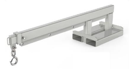
Note: All lift truck attachments affect the safe working load of a lift truck. End users should consult their lift truck supplier to ensure the lift truck is rated for use with these attachments. In the case of a slung load when lifting a jib attachment, the net lifting capacity should be 0.8 times the rating of the lift truck to allow for the swinging load. Please consult your local lift truck dealer
