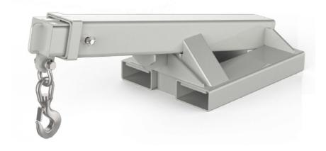
Note: All lift truck attachments affect the safe working load of a lift truck. End users should consult their lift truck supplier to ensure the lift truck is rated for use with these attachments. In the case of a slung load when lifting a jib attachment, the net lifting capacity should be 0.8 times the rating of the lift truck to allow for the swinging load. Please consult your local lift truck dealer.
